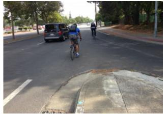
Figure 5: View north on Rengstorff at the north-east corner. Right turn from Central Expressway is a challenge for bicyclists; shallow angle of intersection means that merging motorists must be able to turn their head more than 90 degrees to assess gaps in northbound traffic.
