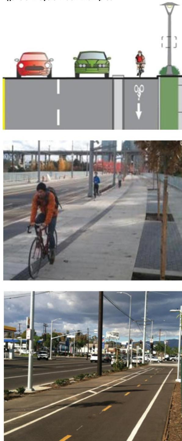
Proposed pedestrian level improvements include wider sidewalks, pedestrian level lighting and median island refuges.
